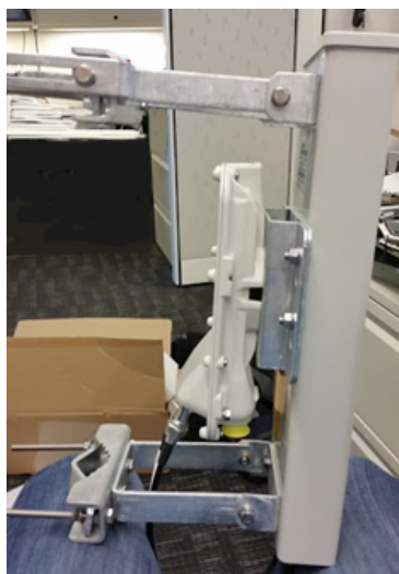
Figure 95: Completed AP and antenna assembly
