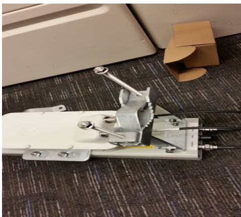
Figure 94: Lower bracket attached to AP antenna
