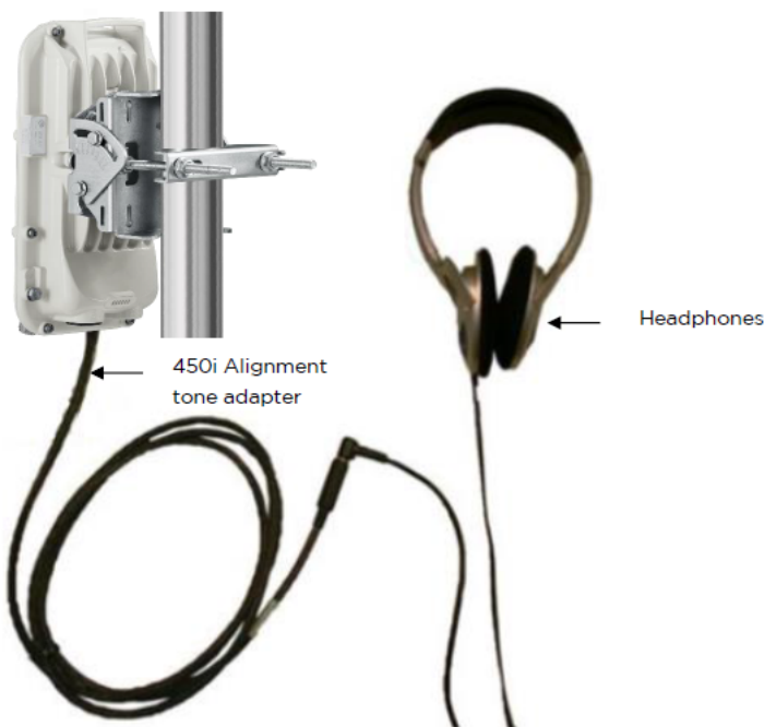
Figure 84: PMP/PTP 450i Series link alignment tone
