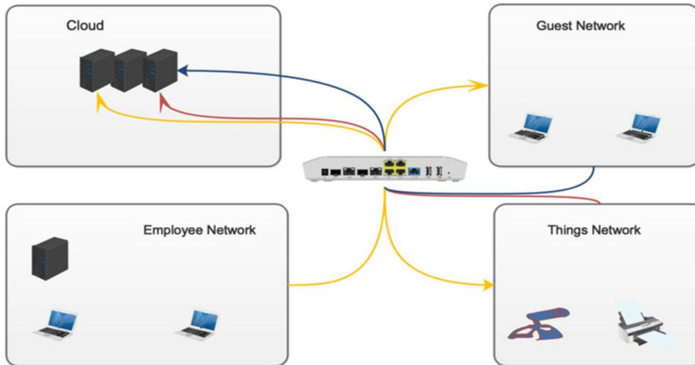
With the help of Radius server on the NSE 3000, users can be authenticated who are connecting to wireless or connecting remotely over VPN. NSE 3000 can function as DHCP server as well as relay agent.
