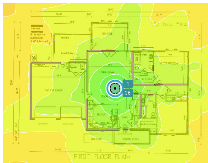
Figure 6 - Wi-Fi coverage for single carriage home
