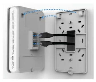
5. Secure e430 to the bracket with a screw at the bottom edge of e430 using standard Torx security screw or standard Philips head screw.
