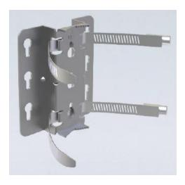
2. Fix the clamp to the pole by applying 9.0 Nm torque.
