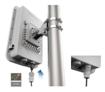
5. Align Radio to required angle by tilting up and down. The maximum radio tilting angle is  $\pm$  40°, with an incremental of 10°.
