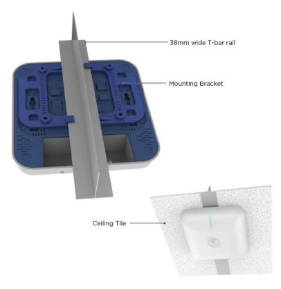
The e410/e600 can be secured to a 38mm ceiling T-bar rail by using the ceiling mount bracket.
