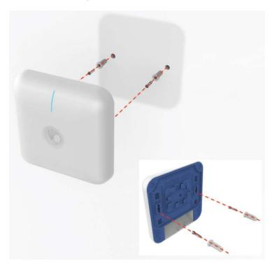
You can mount e410/e600 to any wall by using two screws with corresponding wall anchors. The ceiling mount bracket can be used as a template to align the screws with the unit.
