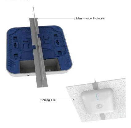
The e410 can be mounted to a 24mm width T-bar rail using the clips built into the underside of the unit.
