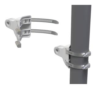
3. Assemble XV2-2T1 (with pole mount holder) to pole mount bracket. Use M12 stud, washer, and M12 nut to secure it by applying 3Nm torque, as shown below.
