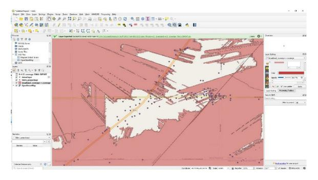
cnHeat provides 1-meter precise coverage predictions based on LIDAR data that meets BDC requirements. Built upon Cambium Networks' expertise in fixed wireless RF planning, propagation, and modeling and integrated with GIS data, cnHeat enables network operators to generate highly accurate RF predictions and offer reliable service with fixed wireless broadband technology.
