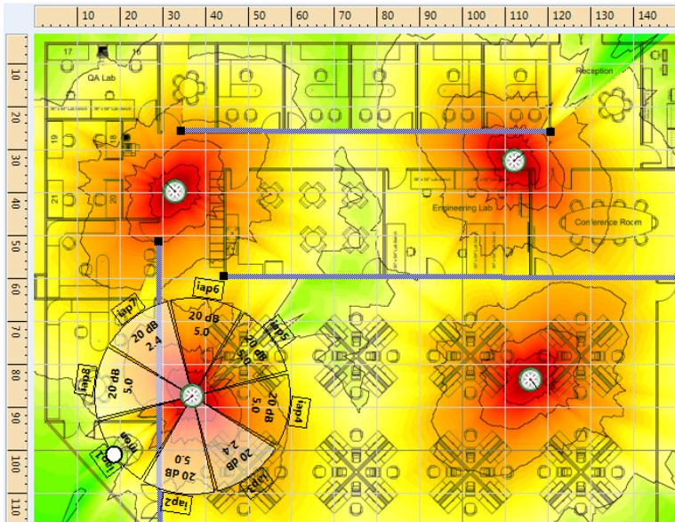
Figure 56. Planning Analysis Display with RSSI Lines
