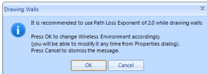
Figure 46. Wireless Environment Path Loss Exponent Warning
