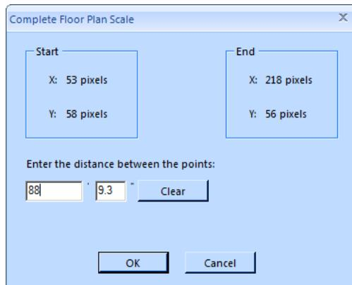
Figure 8. Complete Floor Plan Scale (Calibrate Distance)
