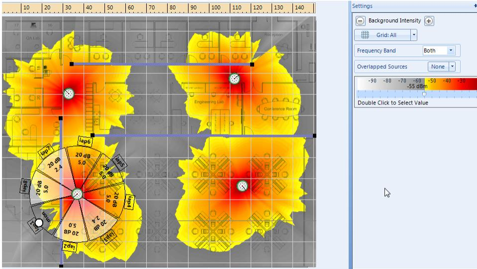
Figure 58. Planning Analysis Display Showing Unacceptable Signal Strength
