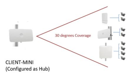
Figure 2-4 CLIENT MINI configuration options
