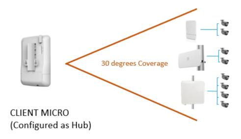
Figure 2-5 CLIENT MICRO configuration options
