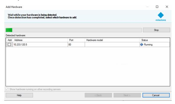
7. The status message will display the results. In case of failure, check and confirm the IP address and the port number is entered correctly. Click the **Next** button to continue.
