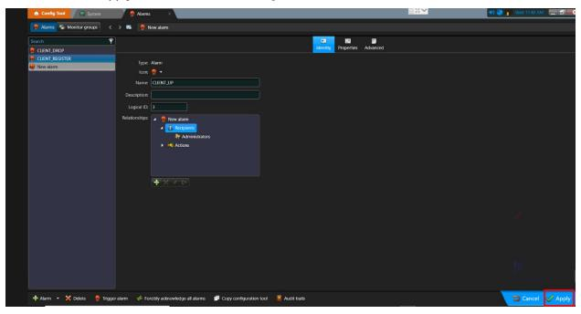
7. The new Alarm has been created and displayed in the left pane. The next step is to link Event message to Alarms.
