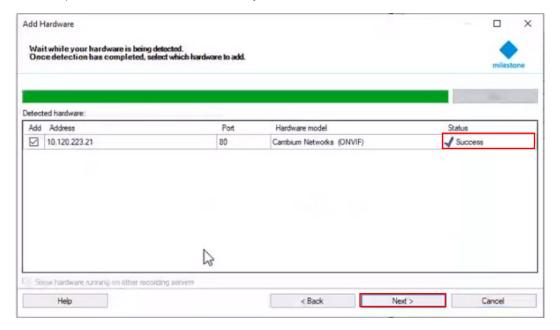
8. The system detects cnVision devices as Cameras. Click the box next to the Camera item to **enable** the device.
