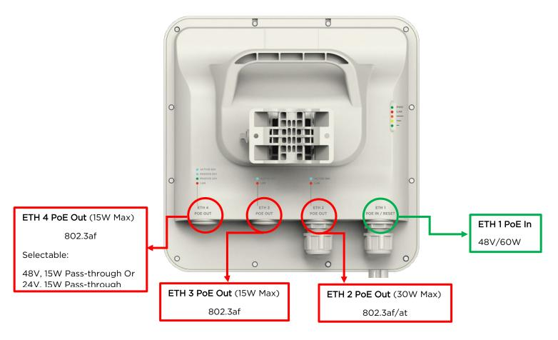
Figure 2-3 CLIENT MAXrp rear interface (PoE ports)
