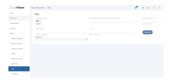
2. Enter the camera's IP address. Click the **Start Ping** button. The ping results will be displayed after the test is complete. If you see replies from the camera such as "Destination Host Unreachable" or "Request Timed Out", the camera may be unavailable for various reasons.
