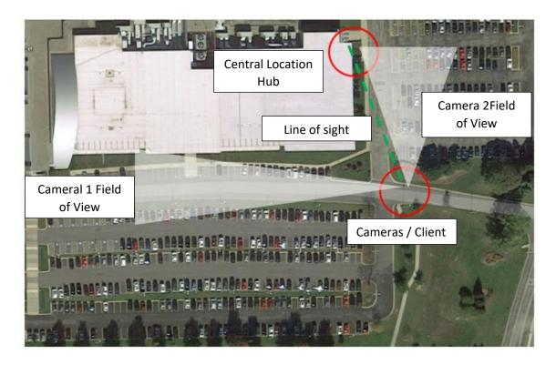
Figure 3-2: cnVision Installation Layout example
