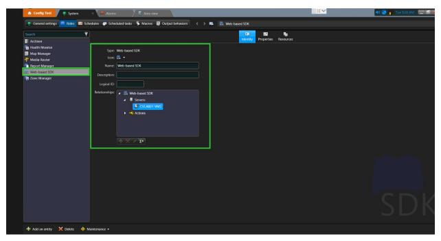
7. Next, click the **Properties** button to access the Port Number. **Note**: This information will be required to configure the VMS settings on the hubs and clients connecting to this system.
