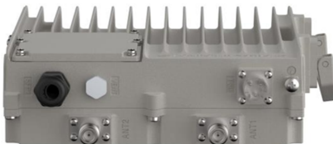
Figure 4: 2 GHz cnRanger 220 RRH front view
