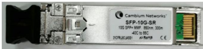
Figure 11: 10Gbps Optical SFP+ transceiver module
