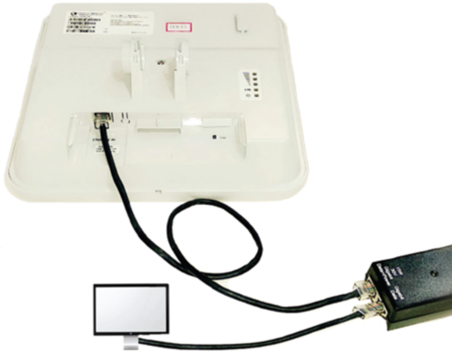
Figure 28: Installation of Tyndall 101 to PoE adapter
