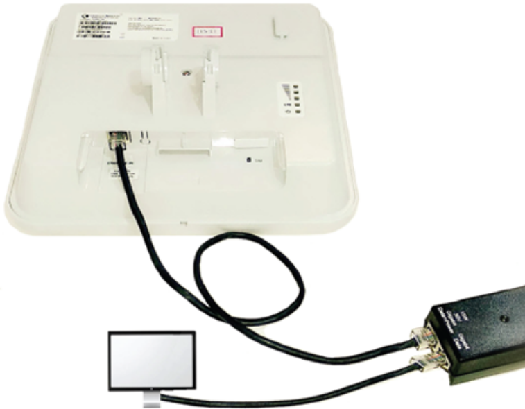
Figure 1: Installation of Tyndall 101 to PoE adapter
