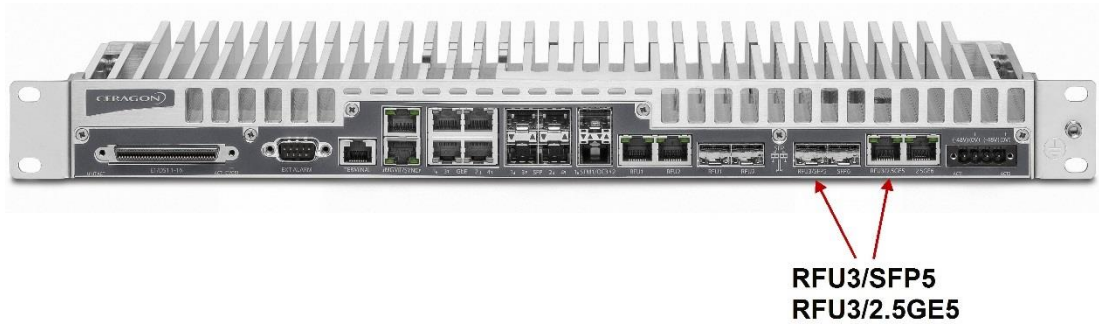
Figure: RFU3/SFP5 and RFU3/2.5GE5 Combo Port
