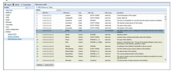
The MIB Reference Table is customized to the type of PTP 820 product you are using. There are three separate versions of the MIB Reference Table:
