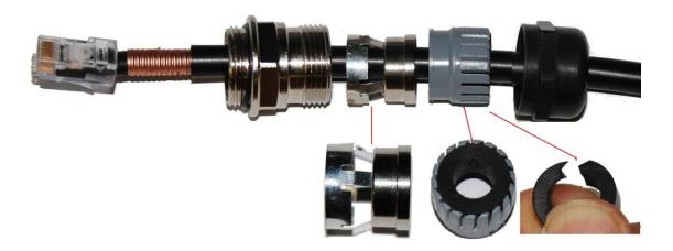
2 Fit the parts into the body and lightly screw on the gland nut using 24 mm (0.9 in) wrench/spanner (do not tighten it):
