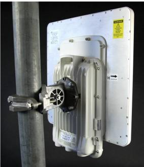
The PTP 700 Connectorized ODU is intended to work with separately mounted external antennas. External antennas generally have higher gains than the integrated antennas, allowing the PTP 700 to cope with more difficult radio conditions.
