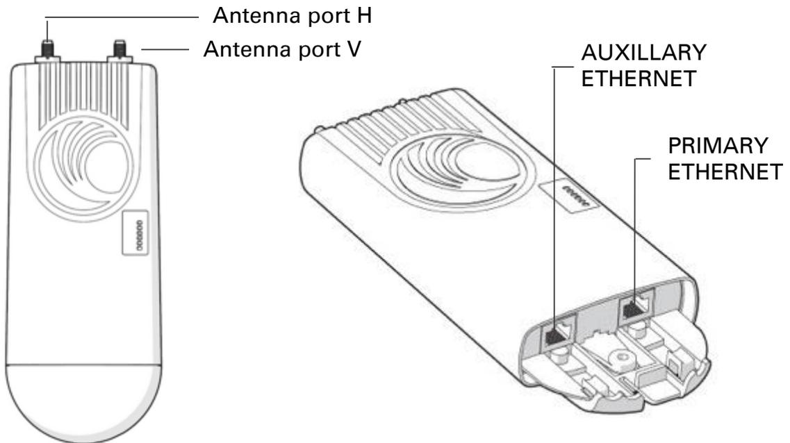
Table 30 ePMP 1000 Connectorized radio interfaces
