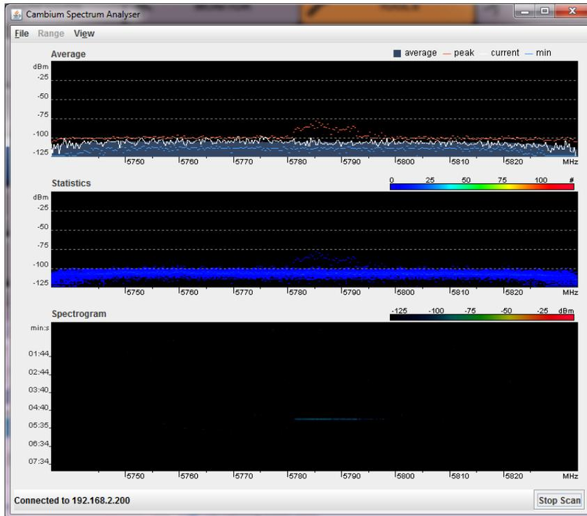
Display of the average, peak, current, and minimum power levels for the configured range
