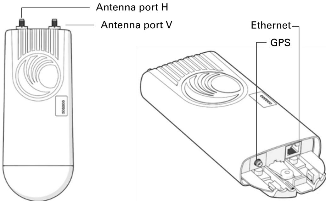
**Table 13** ePMP 1000 Connectorized Radio with Sync interfaces
