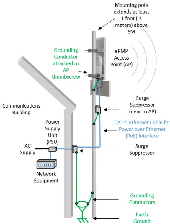
Figure 4 AP Cabling Diagram
