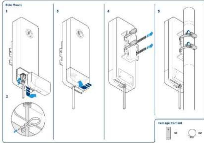
The Force 130 module is designed to be pole-mounted using the mounting straps provided in the box with the radio.
