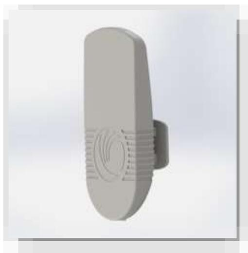
The integrated ePMP 1000 module is a self-contained transceiver unit that houses both radio and networking electronics. An ePMP 1000 integrated unit may function as an Access Point (AP) or a Subscriber Module (SM) in a Point-To-Multipoint (PMP) or in a Point-To-Point (PTP) network topology.
