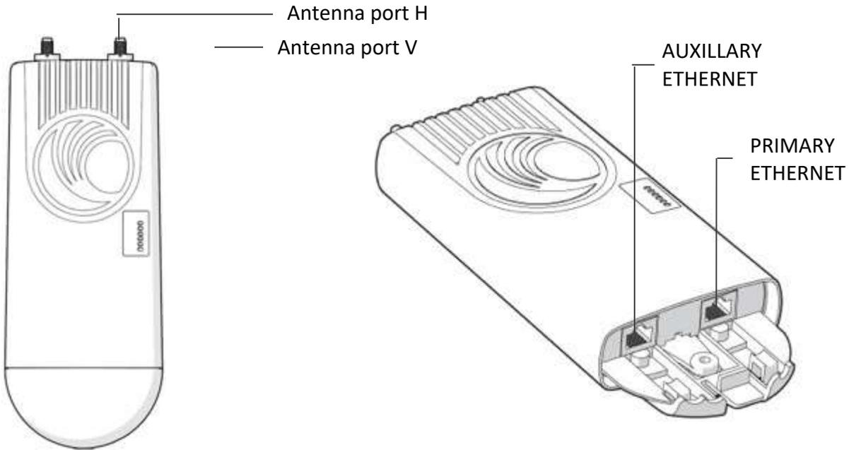
**Table 30** ePMP 1000 Connectorized radio interfaces
