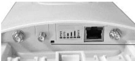
ePMP 2000 Access Point with Intelligent Filtering and Sync Reset Button
