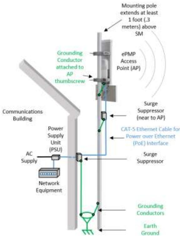
Figure 4 AP Cabling Diagram
