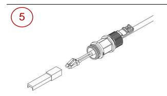
Connect the fibers to the SFP transceiver. Listen for the "click" to ensure that they are fully inserted.
