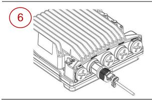
Secure the cable to the gland using a tie wrap.
