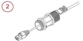
Insert the CAT5E cable into the gland cap and into the rubber gland.
