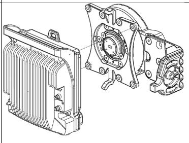
If necessary, change the antenna polarization by rotating the unit in accordance with the relevant antenna installation guide.
