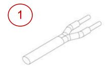
Strip off 45 mm from the cable jacket and expose 10 mm at the edge of each of the two wires.
