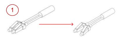
Split the connector into two separate LC connectors, one for each fiber.
