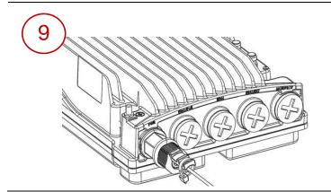
Secure the cable to the gland using a tie wrap.
