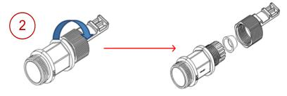
Remove the gland cap and rubber from the gland body
