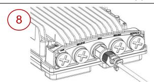
Secure the cable to the gland using a tie wrap.
