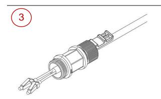
Slide the gland cap into the cable.
