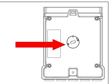
Mount the PTP 820S on the antenna using the four M8 captive screws and washers that are supplied, assembled, in the PTP 820S, and tighten the screws.
