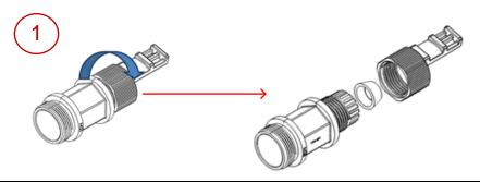
Remove the gland cap and rubber from the gland body
