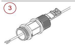
Insert the power cable into the gland.
