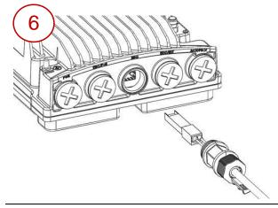
Remove the tie wrap securing the cable to the gland and connect the connector into the PTP 820S connector.
