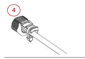
Secure the cable to the lip of the gland using a tie wrap. This is to prevent the cable from slipping from the gland when raising the cable to a radio unit on a tower.
