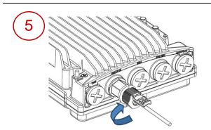
Hand-tighten the gland to the radio unit until there is full contact between the gland and the radio unit and handtighten the gland cap.
