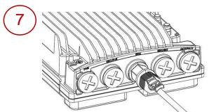
Hand-tighten the gland to the radio unit until there is full contact between the gland and the radio unit and hand-tighten the gland cap.
