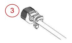
Secure the cable to the lip of the gland using a tie wrap. This is to prevent the cable from slipping from the gland when raising the cable to a radio unit on a tower.
