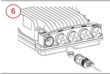
Plug the power cable with connector into the PTP 820S power connector.
