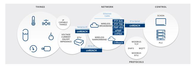
For operators with existing IP networks, the cnReach IO expander can be used to migrate the traditional "Things" to IIOT architecture. Operators can also deploy PTP820, PTP700, PMP450, etc. to transport the IIOT traffic if line-of-sight wireless broadband is feasible. In non-line-of-sight deployments, the cnReach narrow band radio can be used to enable the IIOT data transport.
