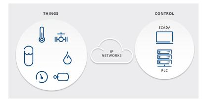
The architecture above works for green field deployment, meaning that if an operator wants to move to IIOT, they would need to upgrade all their existing sensors and other controllable equipment (machines) to IP capable "things". This would be expensive. A more practical approach would be to reuse existing "things" by connecting them with IIOT adapters, and migrate to IIOT gradually.
