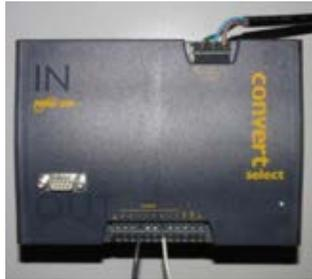
**Figure 31** 56 VDC power supply DC connection
