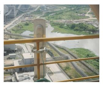
Installation was simple and straightforward. Because there were multiple cameras at the pole locations, two FE ports were required for connecting the cameras to the radios. "Based on the design model, the auxiliary port on the ePMP SM helped to eliminate the need for a switch at each pole and also provide relay to cover blank spots," says Wajapey.
